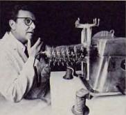
Paint shaker is switched on. The torture begins. 335 vibrations a minute.
